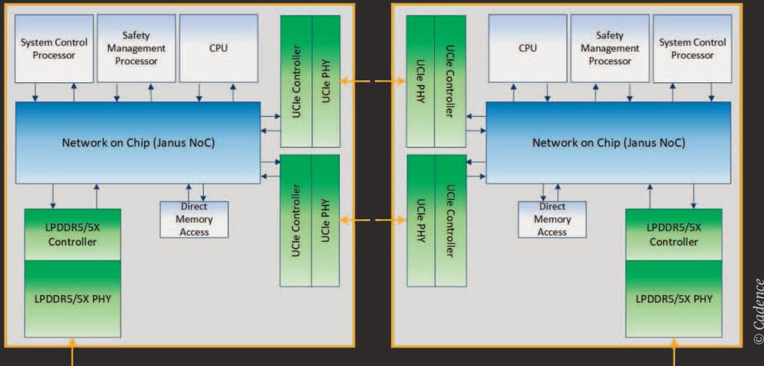
This diagram shows how two system chiplets can be integrated on the same package
